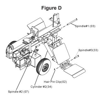
The Spindles are used to assemble and connect the Log Lift (01) to the main unit - See Figure D.
